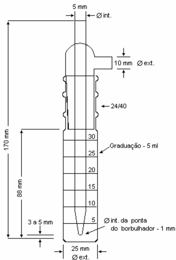
FIGURA 1 - Borbulhador (Midget-impinger)
